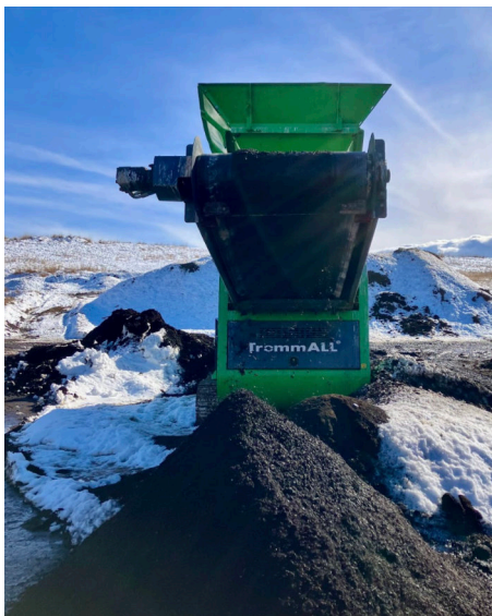
Screening compost at Story Mill Convenience Site Credit: Happy Trash Can
