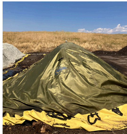
SG Mobile® GORE® Cover aerated composting system Credit: Happy Trash Can
