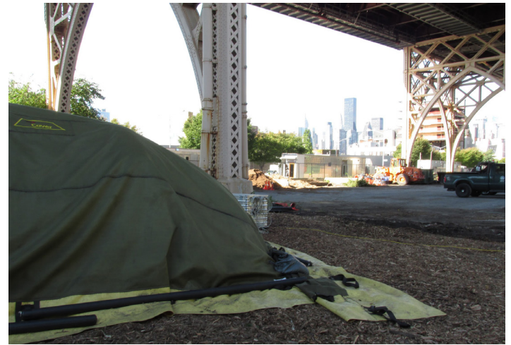
▲ The NYC Compost Project hosted by BIG Reuse located under the Queensboro Bridge uses a GORE® cover to convert an otherwise aerated static pile into an in-vessel composting system. Source: Institute for Local Self-Reliance.
