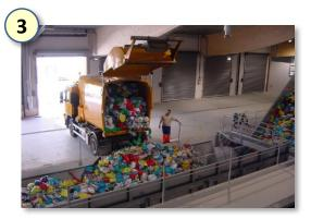
Materials are separated at transfer station. Automated optical sort systems are available to sort bags.
