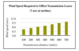
Overall, transmission and array losses increase the cost of power production. A project 500 miles distant would cost about 1.8 cents/kWh more than a local project. Higher wind speeds could lower generation costs to offset or exceed these higher transmission-related costs. A wind speed 5.3 percent higher would be needed to offset a 500 mile trip.
