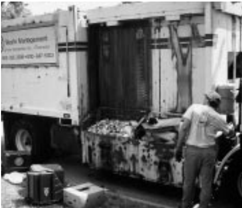
WMI collector loading recyclables into side-loading 40-cubic-yard split packer truck
