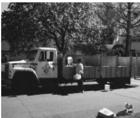
Three-person DPW crews collect recyclables in a five compartmented Eager Beaver truck. Paper is collected separately in a packer truck.
