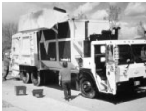
Two-person crews dual-collect recyclables and trash using specially designed semi-automated one-pass trucks.
