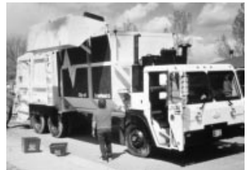
In Loveland, two-person crews use dual-collection vehicles to collect recyclables and trash at the same time.
