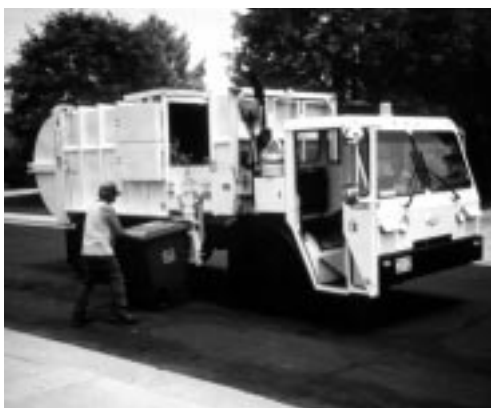
In Loveland, Colorado, residents can pay $4 a month for weekly curbside yard trimmings collection. They receive a 90-gallon roll cart. Here, a 16-cubic-yard semi-automated truck empties a cart.
