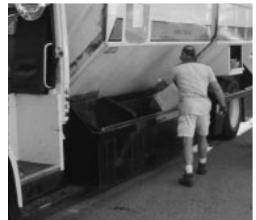
USA Waste collector unloading recyclables into side-loading vehicle
