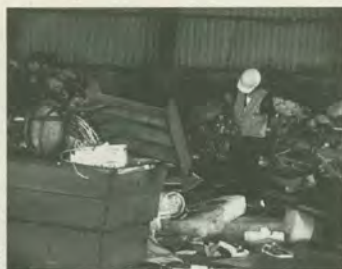
Salvager holding chairs at transfer station. The salvager's job is to find items that are good as is, can be repaired, or in any event can be sold. He or she has to recover them before the loader operator pushes the material into the big pile.
