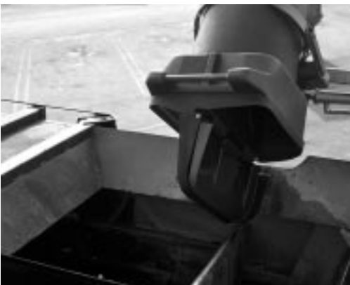
110-split containers are automatically emptied into hopper of split compactor trucks.
